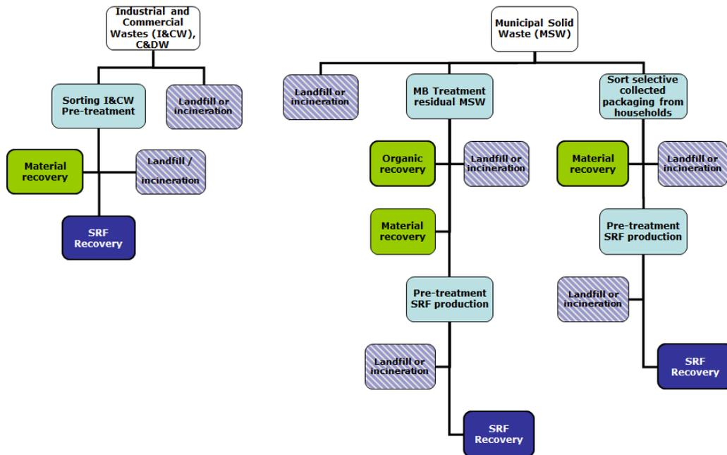
**Schematic process of the production of SRF**
